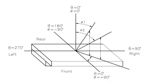
NOTE2: Definition of viewing Angle Range:  $\Delta \Phi = |\Phi 2 - \Phi 1|$
