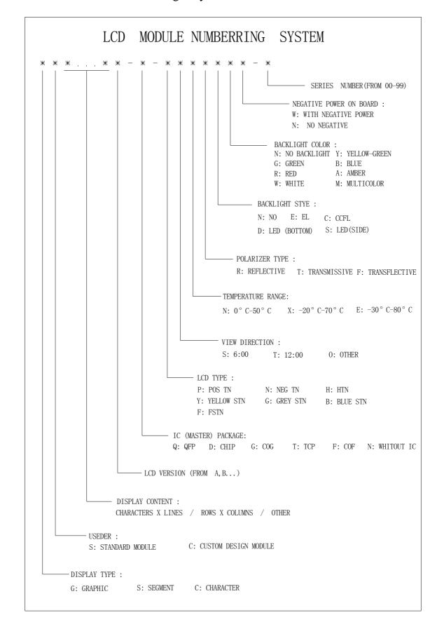
1. LCD Module Numbering System
