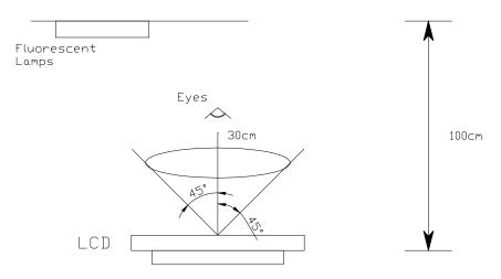
10.4.1.2 When test the model of transmissive product must add the reflective plate.
