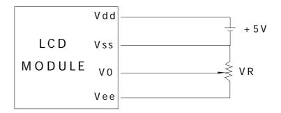
Vdd-V0: LCD Driving Voltage
