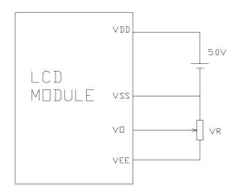
VDD-VD: LCD driving voltage VR: 10K-20K
