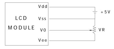
Vdd-V0: LCD Driving Voltage
