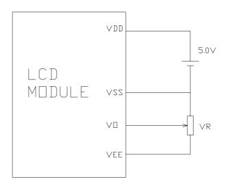
VDD-VD: LCD driving voltage VR: 10K-20K
