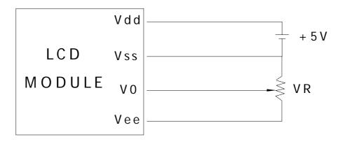
Vdd-V0: LCD Driving Voltage
