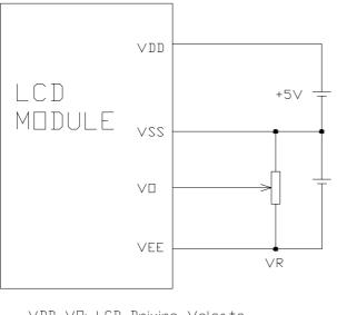
VDD-VD: LCD Driving Volgate VR: 10K-20K
