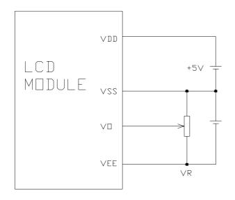
VDD-VD: LCD Driving Volgate VR: 10K-20K
