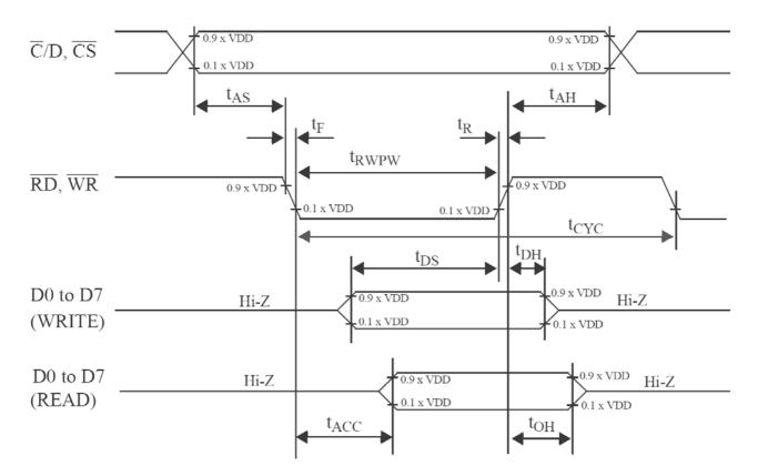
AC timing for interface with a 80-type microcontroller at VDD=5volts. Ta = -20 to 75 deg. VDD =  $5.0V \pm 10\%$ ;VSS=0V;
