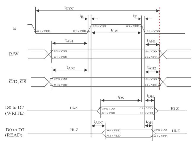
AC timing for interface with a 68ype microcontroller at VDD=5volts. Ta = -20 to 75° C, VDD = $5.0V \pm 10\%$ ;VSS=0V.
