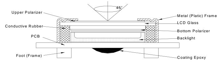
View Angle: with in 45° around perpendicular line.
