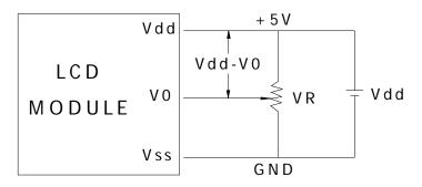
Vdd-V0: LCD Driving Voltage
