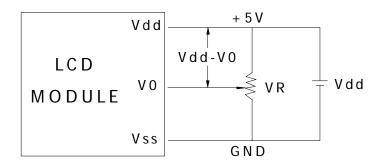
Vdd-V0: LCD Driving Voltage
