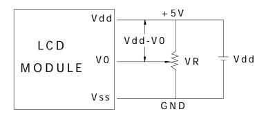
Vdd-V0: LCD Driving Voltage
