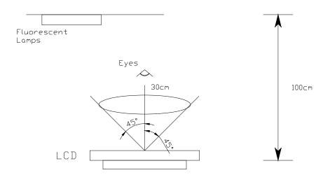
12.4.1.2 When test the model of transmissive product must add the reflective plate.
