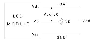
Vdd-V0: LCD Driving Voltage
