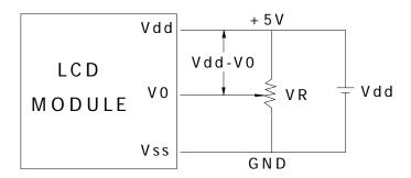
Vdd-V0: LCD Driving Voltage
