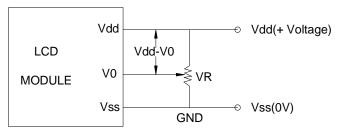
Vdd - V0: LCD Driving Voltage
