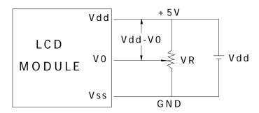
Vdd-V0: LCD Driving Voltage
