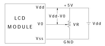
Vdd-V0: LCD Driving Voltage
