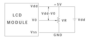
Vdd-V0: LCD Driving Voltage
