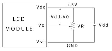
Vdd-V0: LCD Driving Voltage VR: 10K - 20K
