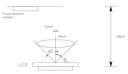
12.4.1.2 When test the model of transmissive product must add the reflective plate.
