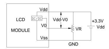
Vdd - V0: LCD Driving Voltage
