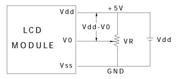
Vdd-V0: LCD Driving Voltage
