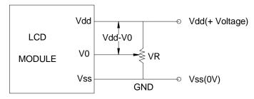
Vdd - V0: LCD Driving Voltage
