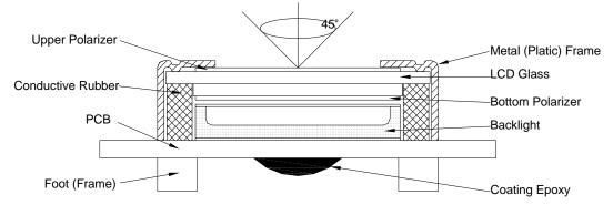
2. View Angle: with in 45° around perpendicular line.
