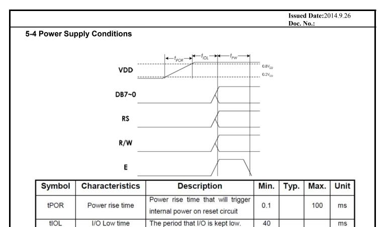
1. During tPOR, VDD noise should be reduced (especially close to 2.0V). Otherwise the Power-ON-Reset function might be triggered several times and maybe cause unexpected result.
