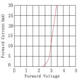
2. Forward current VS Forward Voltage
