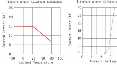
2. Forward current VS Forward Voltage
