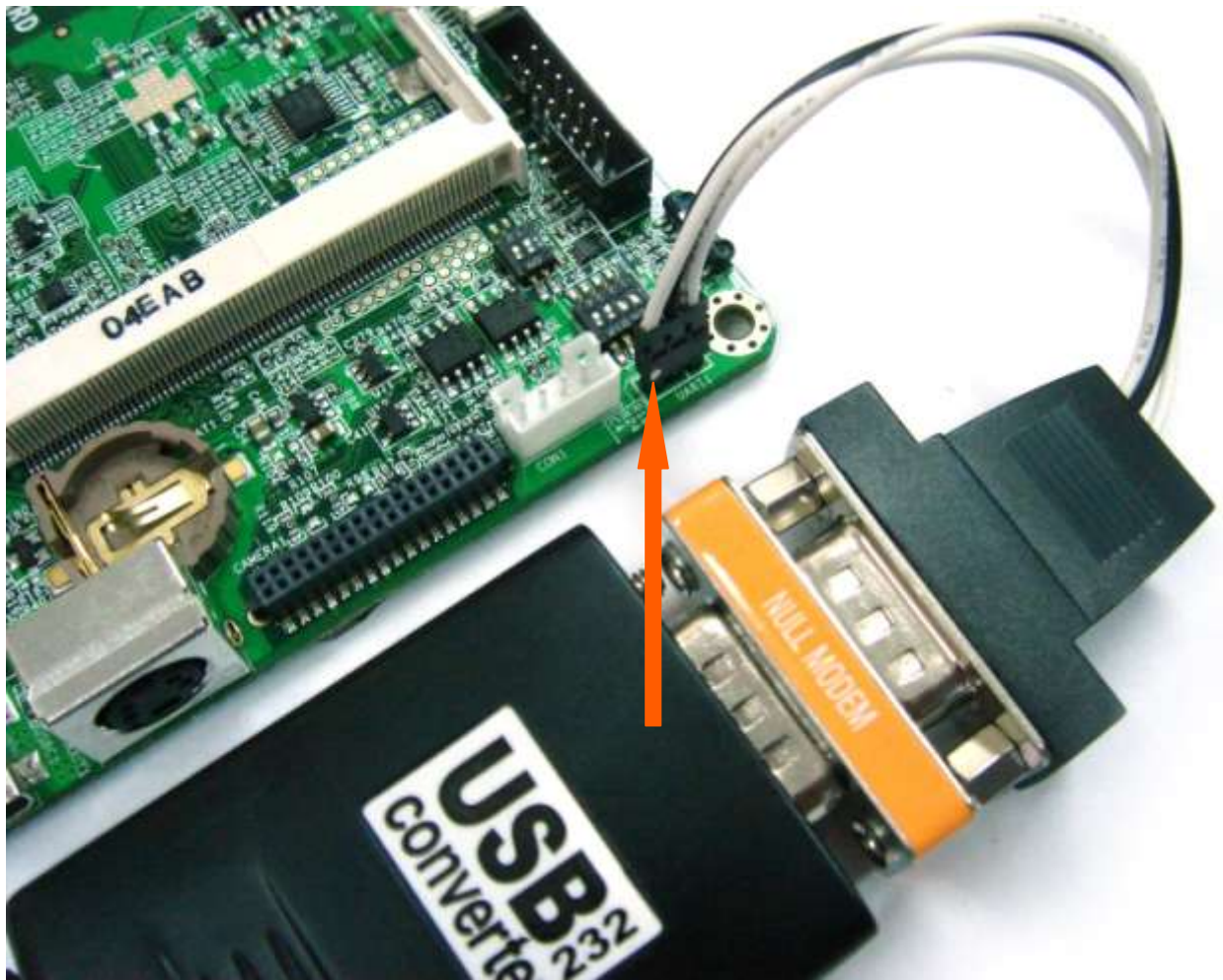
Figure 37: The cable (RS-232 to USB) with null-modem-block connected to the UART1 (5) connector (see orange arrow for position of the white dot (note: turned 180 degrees))
