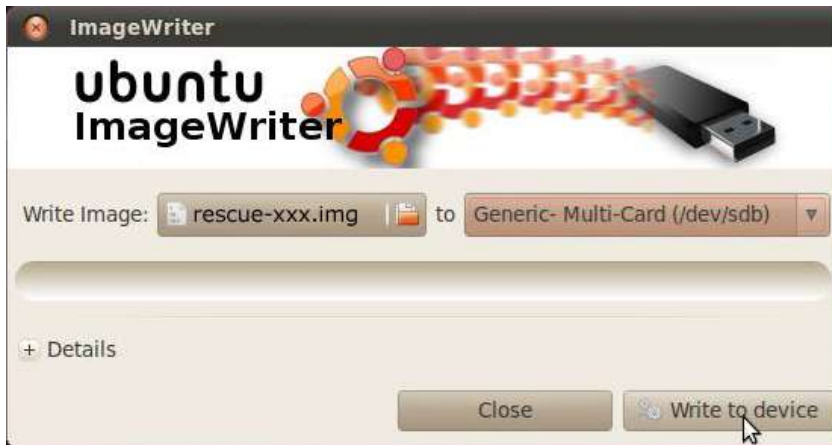
Figure 29: Select the downloaded image and destination (SD-card in your computer), click write to device
