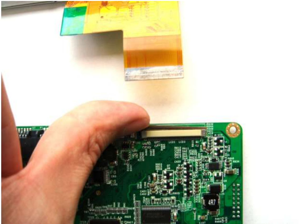
Figure 5: Step 2a - Pull the connector at the bottom side of the Tsunami baseboard sideward open with your nail.
