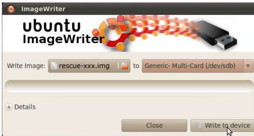
Figure 39: Select the downloaded image and destination (SD-card in your computer), click write to device
