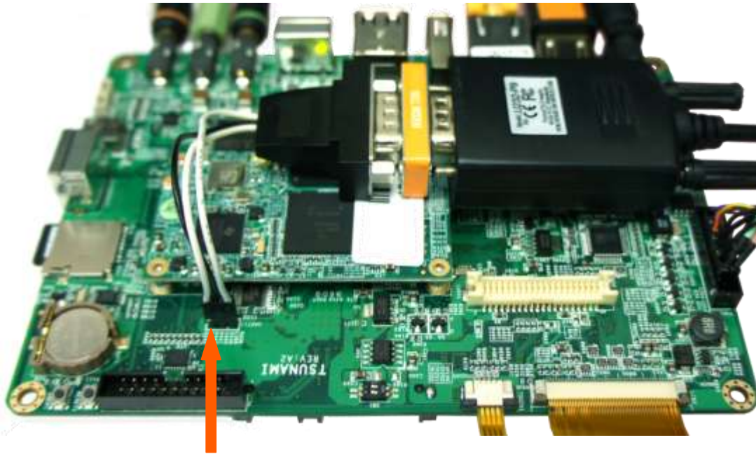
Figure 47: The cable (RS-232 to USB) with null-modem-block connected to the debug connector (see orange arrow for position of the white dot (note: turned 180 degrees))
