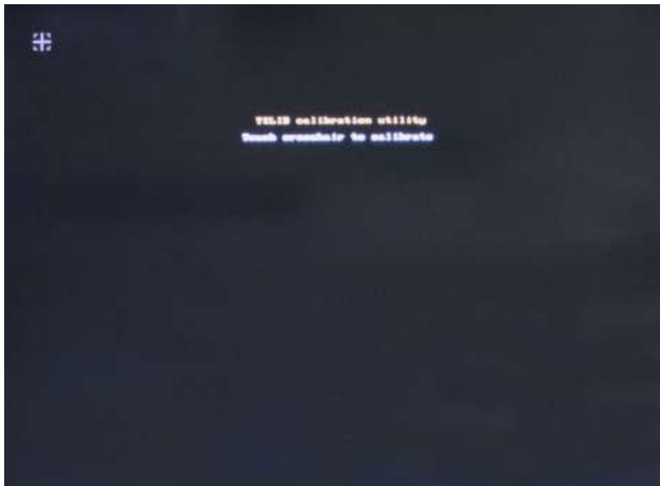
Figure 55 : touch the crosshairs on the screen. After Calibration it will reboot to store the settings
