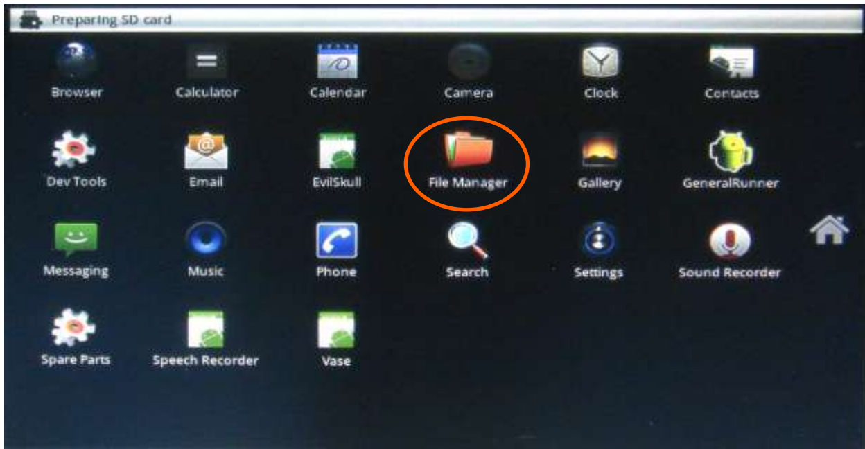
Figure 61: Use the “left arrow” button on the USB-keyboard to go BACK to the main menu. Insert a micro-SD card with the application on it in the baseboard. In the top left it will show “preparing SD card” which will disappear after the SD-card is detected. Press on the “File manager”. (If you do not have FileManager or Astro then go to the next paragraph 11.2)
