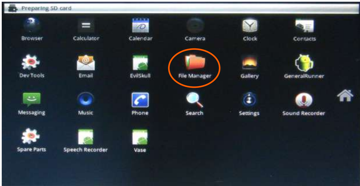
Figure 51: Use the “left arrow” button on the USB-keyboard to go BACK to the main menu. Insert a micro-SD card with the application on it in the baseboard. In the top left it will show “preparing SD card” which will disappear after the SD-card is detected. Press on the “File manager”. (If you do not have FileManager or Astro then go to the next paragraph 11.2)
