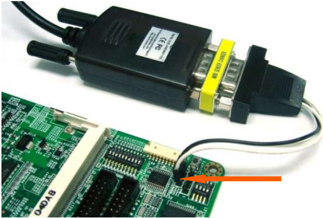
Figure 37: The cable (RS-232 to USB) with yellow mini-gender-changer-block connected to the UART1 connector of the THB-3517 HMI baseboard (see arrow for position of the white dot)
