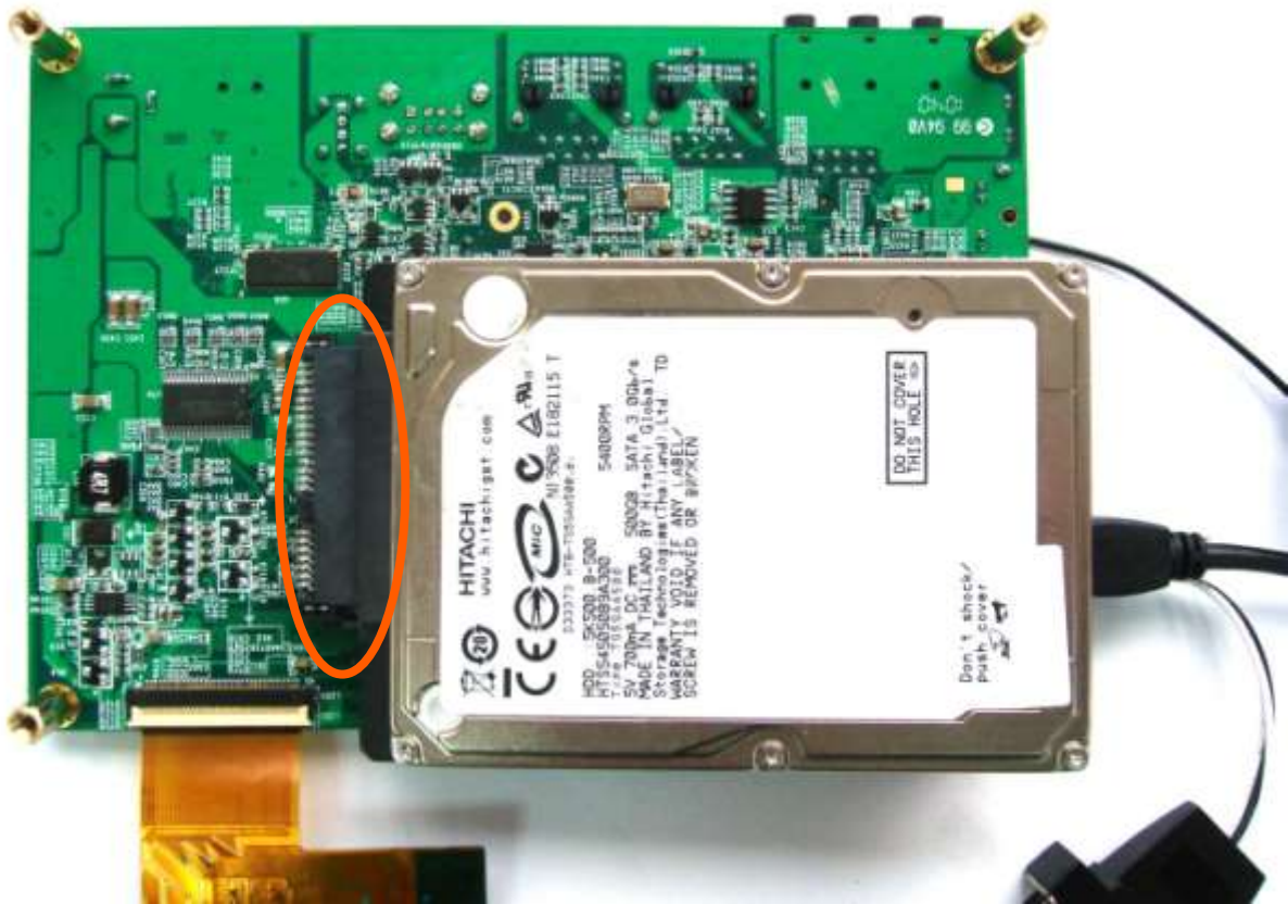
Figure 15: Step1 – Place the 2.5” hard disk in the connector as shown above (you will need to remove one spacer in the bottom right corner).
