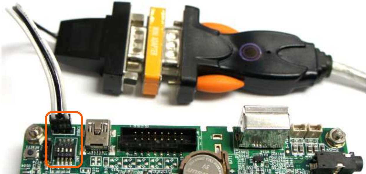
Figure 35 : The Null-modem connected to the UART1 connector Twister baseboard (For debugging the dipswitch (SW2) pin 1 and 2 should be “ON”)
