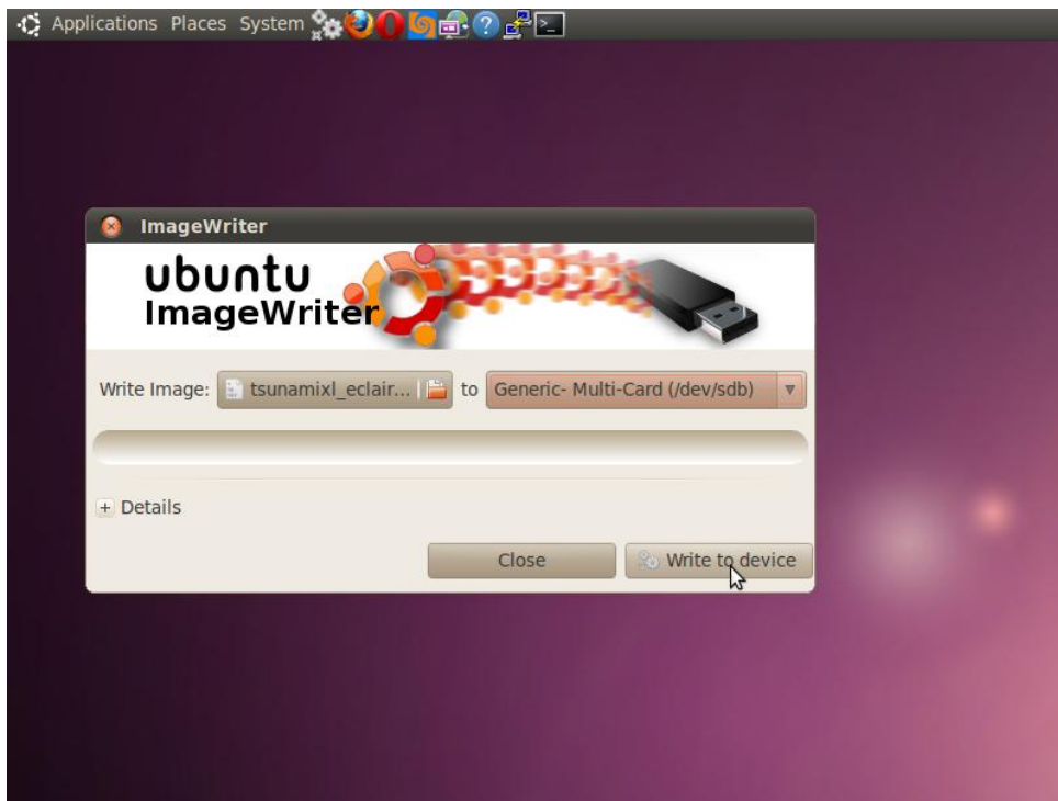
Figure 19: (plug the SD-card with an adapter into your computer). Select image and destination (SD-card), click write to device
