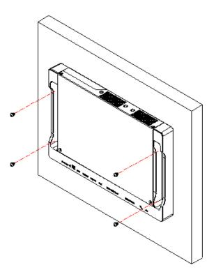
You can install SI-38 on plastic (LCD monitor), wood, drywall surface over studs, or a solid concrete or metal plane directly. Ensure the installer uses at least four M3 length 6mm screws to secure the system on wall. Six M3 length 6mm screws are recommended to secure the system on wall.
