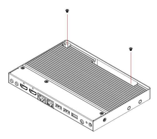
You can install SI-22 on plastic (LCD monitor), wood, drywall surface over studs, or a solid concrete or metal plane directly. Ensure the installer uses at least two M3 length 6mm screws to secure the system on the wall. Four M3 length 6mm screws are recommended to secure the system onto the wall.
