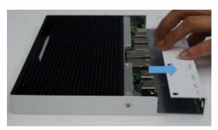
2. Push the WIFI module into the slot. Screw two screws to secure the module in the slot.
