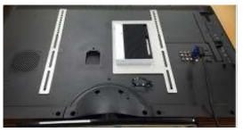
3. Install the TV mounting black bracket on the SI-102-424 silver-color mounting bracket.
