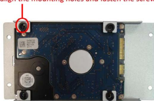
4. Connect SATA power cable and SATA signal cable. Make sure the cables are well connected. Fastener hard drive cover screws.
