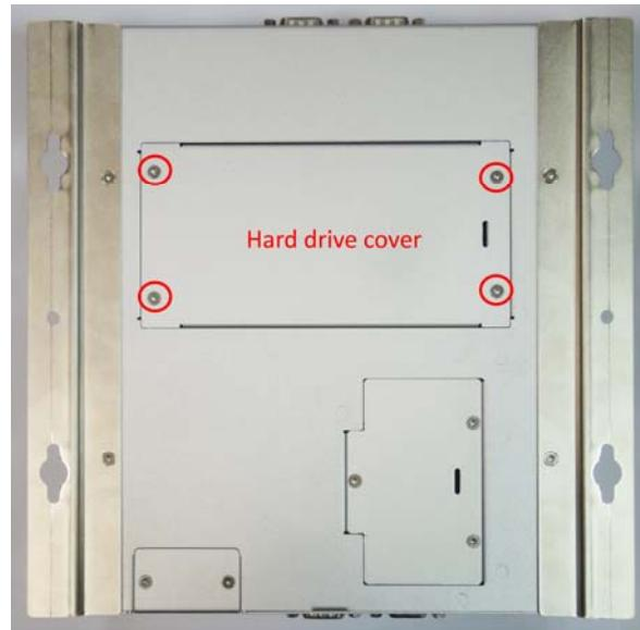
2. Take off the cover. The cover is used to hold a SATA hard drive.
