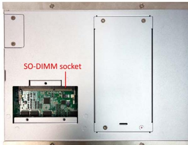
3. Insert the module into the socket at an approximately 30 degrees angle. Apply firm even pressure to each end of the module until it slips into the socket. The gold-plated connector on the edge of the module will almost completely disappear inside the socket
