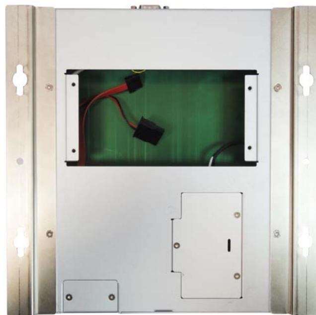
3. There are 4 screws in the accessory packet. Slide the hard drive into the hard drive cover, align the mounting holes and fasten the screws
