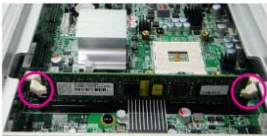
The retaining clips lock onto the module and the memory modules are secured in place.
