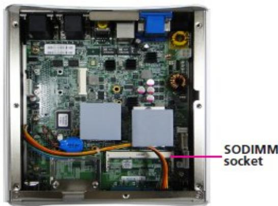
Step 2: Align the notch on the memory module and the socket slot, and insert the memory module until the connectors fully inserted.
