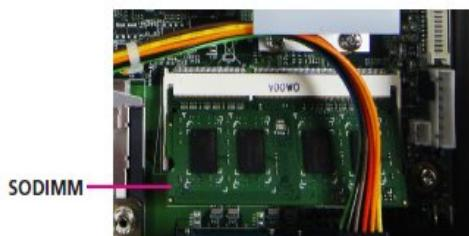
Step 3: Press the module down and then lower it down in place. Press the module by using the edges of the module.
