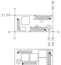
J1 J2: COM3/4/5/6 Serial Ports J1 - COM3/4 pin-header connector. PIN1~PIN10 COM3 PIN11~PIN20 COM4 J2 - COM5/6 pin-header connector. PIN1~PIN10 COM5
