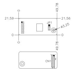
CN1: LPC I/F connectors Package list Nylon Nut x 1 Screw x 2 Washer x2 This page is intentionally left blank.
