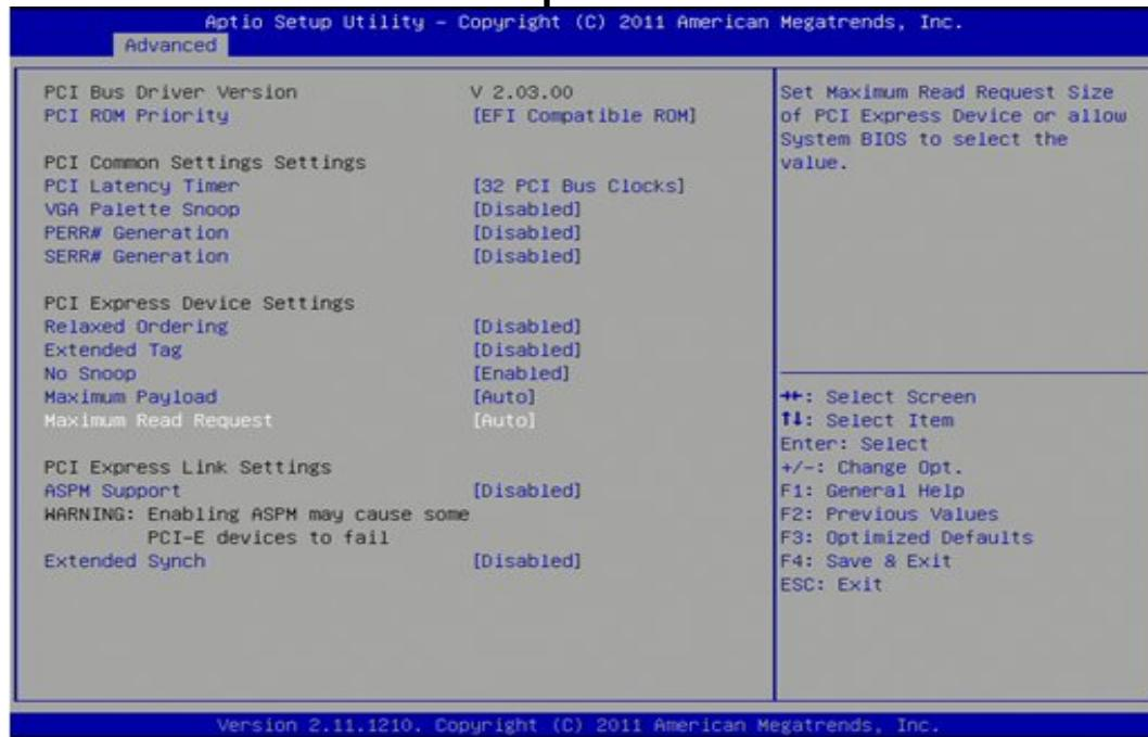
Select this option to set the Maximum Read Request function (Auto).This setting determines the largest read request any PCI Express device can generate. Reducing the maximum read request size reduces the hogging effect of any device.
