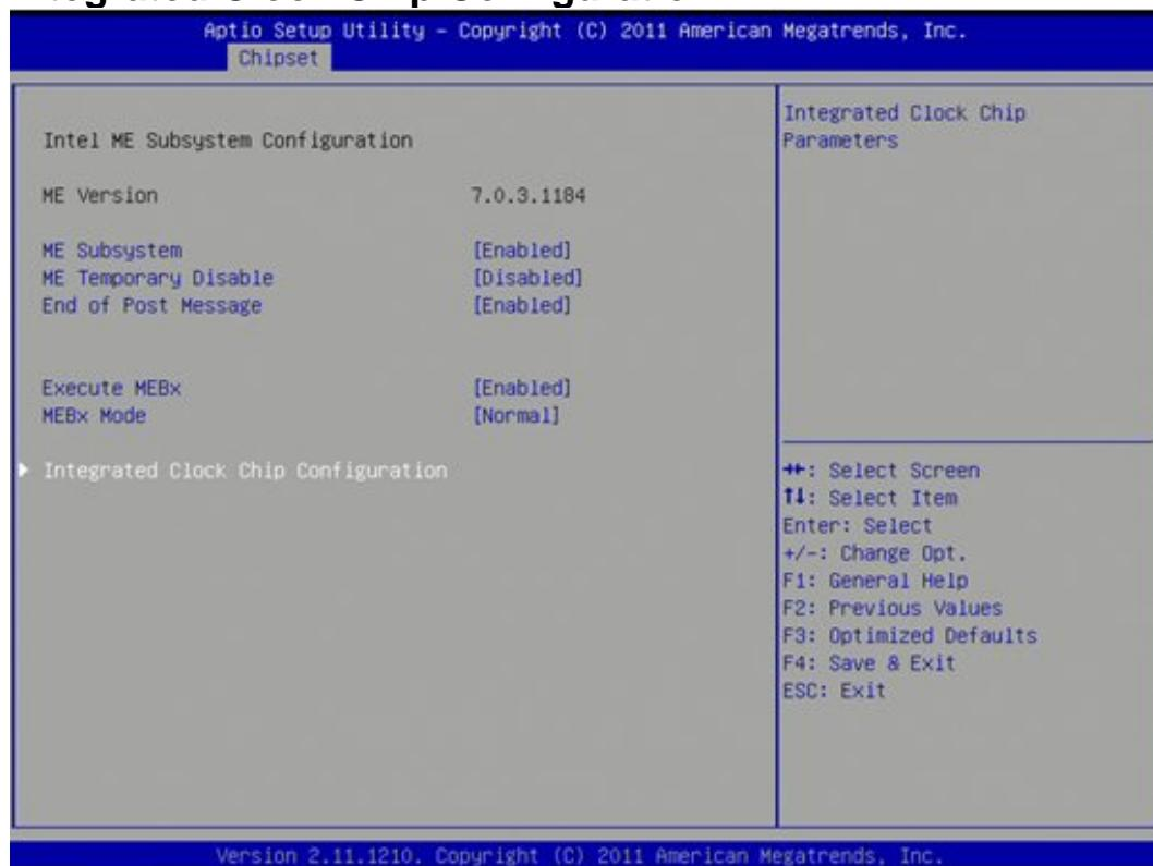
Select this option to set the Integrated Clock Chip Configuration parameters. The Integrated Clock Chip Configuration menu can be accessed to set the overclocking profiles on the BIOS. Performance Tuning can be accessed to adjust the settings in the CPU Configuration and Chipset Configuration submenus. In Turbo mode, the IA Core Current, the TDP, the EIST and Turbo mode can be controlled. The Chipset menu controls the memory timings and graphics configuration.
