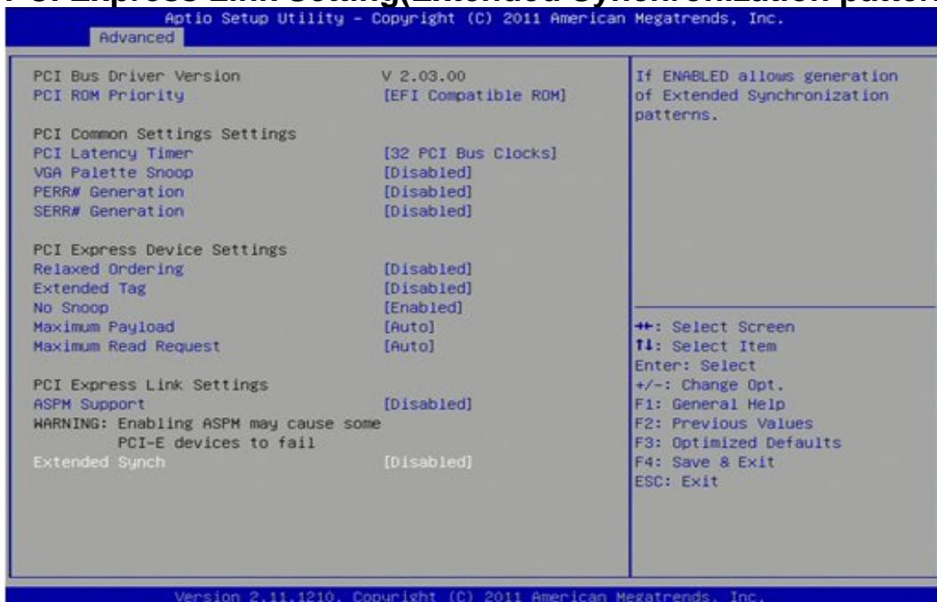
Select this option to enable or disable the Extended Synchronization function (Disabled).If this setting is enabled, the system allows generation of extended synchronization patterns.
