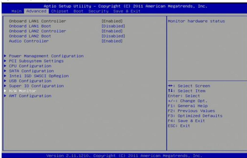
Select this option to set the Hardware Monitor settings. The Hardware Monitor reads out all accessible hardware sensors. Depending on the type of available sensors, the following data can be accessed:
