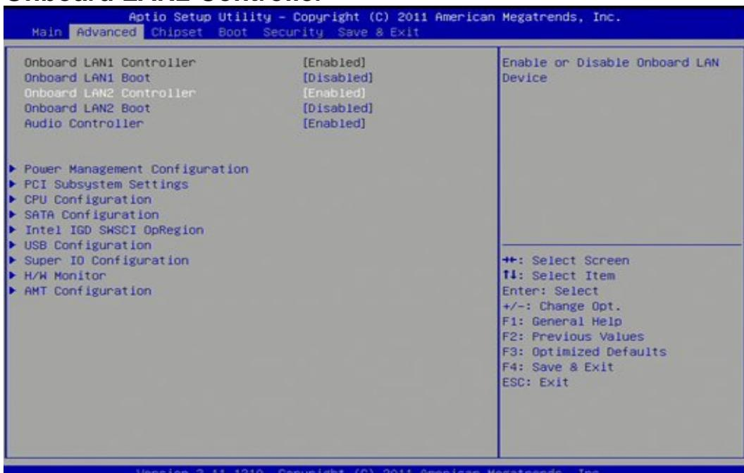
Use this setting to enable or disable the onboard LAN2 (Enabled).
