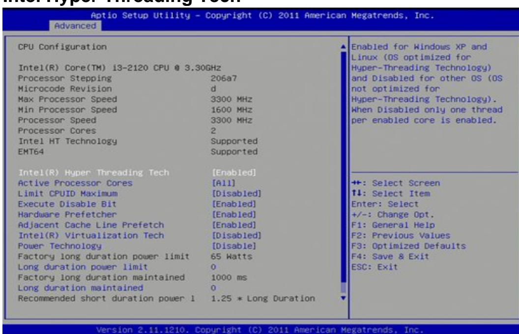
Select this option to enable or disable the Intel Hyper Threading technology (Enabled).
