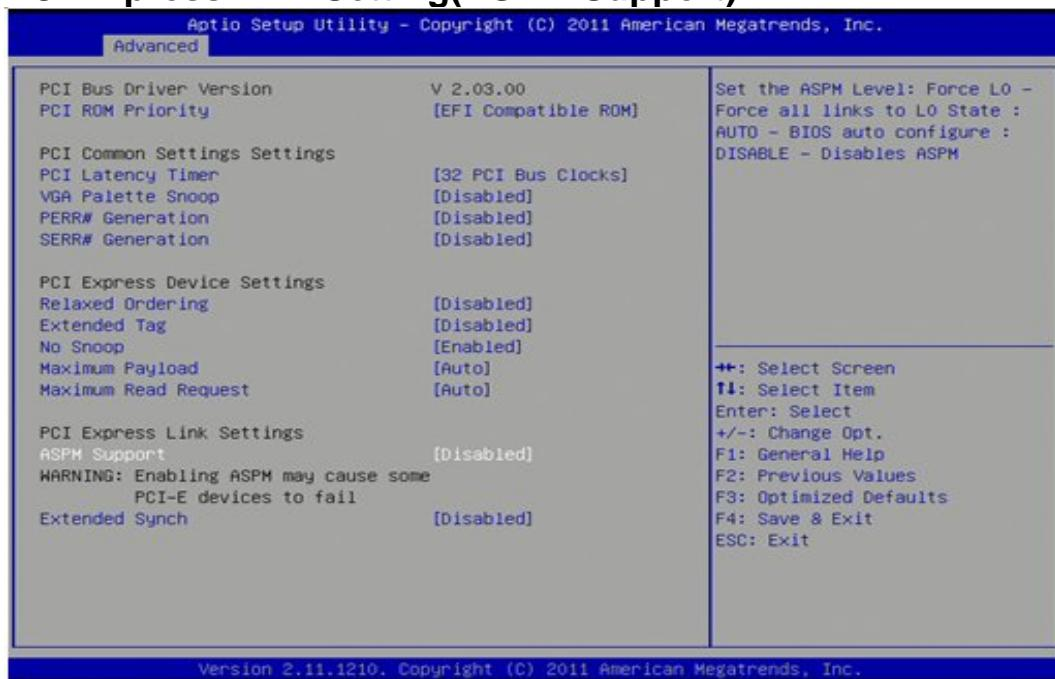
Select this option to enable or disable the ASPM Support function (Disabled).The PCI Express ASPM defines a protocol for PCI Express components in the D0 state to reduce link power.
