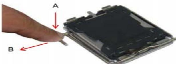
2. Lift and rotate the load lever to unlock the load plate.
