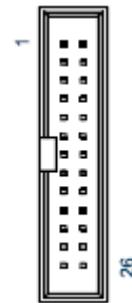
**2.25:DIO1: Digital Input / Output Pin Header**
