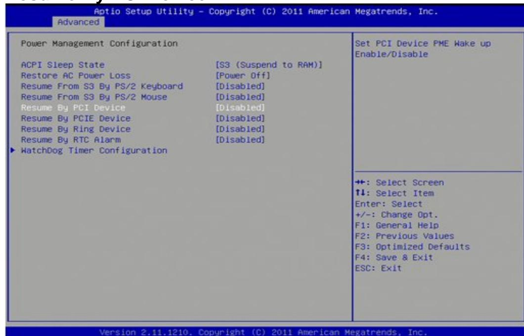
Select this option to disable or enable the PCI device wake up function (Disabled).
