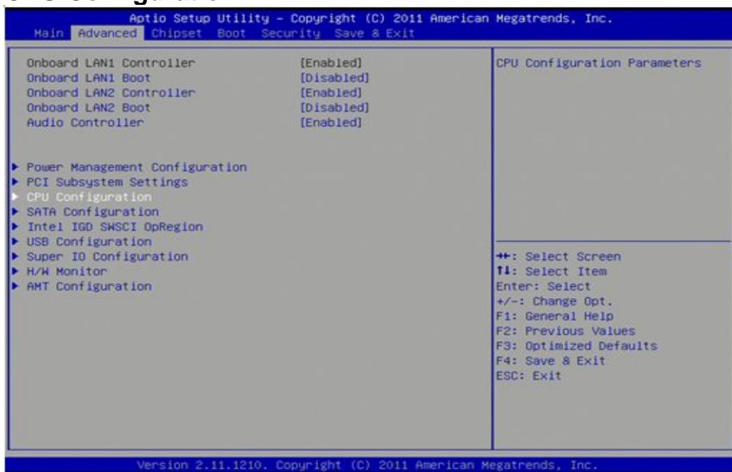
Select this option to set CPU configuration settings, such as: CPU ID, CPU Family, and Clock Speed.
