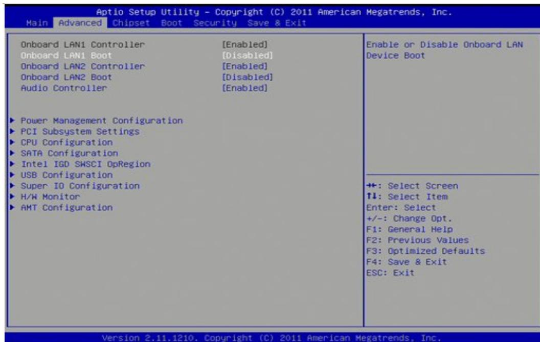
Use this setting to enable or disable the Onboard LAN1 boot (Enabled).
