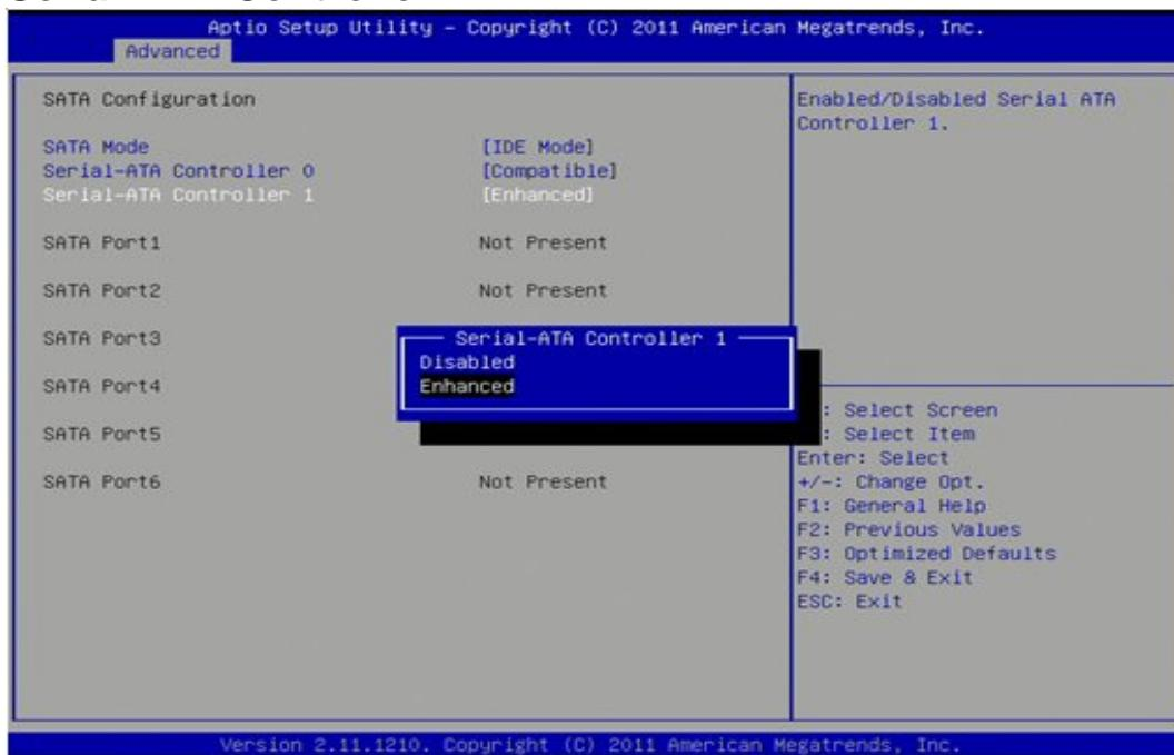
Select this option to set the Serial-ATA Controller 1 function (Enhanced). The following settings are available: Disabled or Enhanced.
