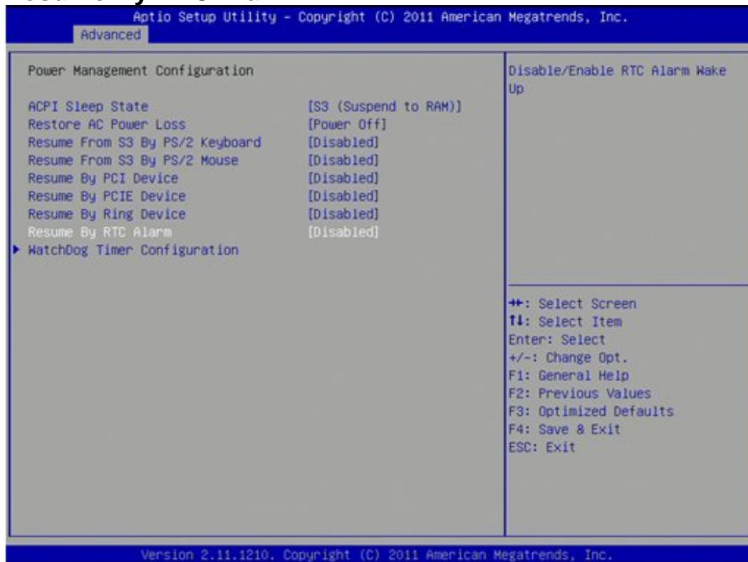
Select this option to disable or enable the RTC Alarm device wake up function (Disabled).
