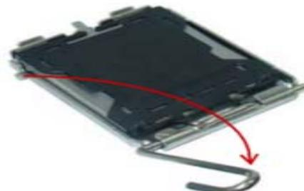
3. Lift the load plate until it is fully open.
