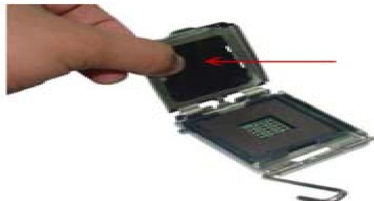
5. Unpack the new processor and remove any protective material.
