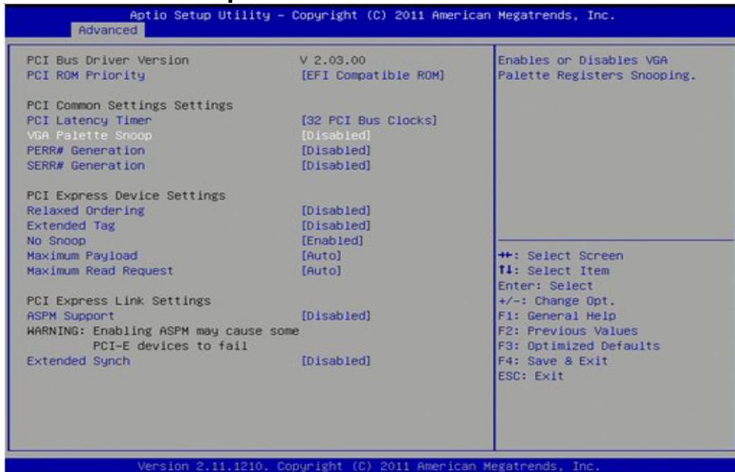
Select this option to enable or disable the VGA palette snoop (Disabled). The VGA Palette Snoop enables PCI cards without a VGA color palette to examine and mimic the video card palette. This feature is required for some MPEG decoder cards, TV cards, and other expansion cards that deal with graphics.
