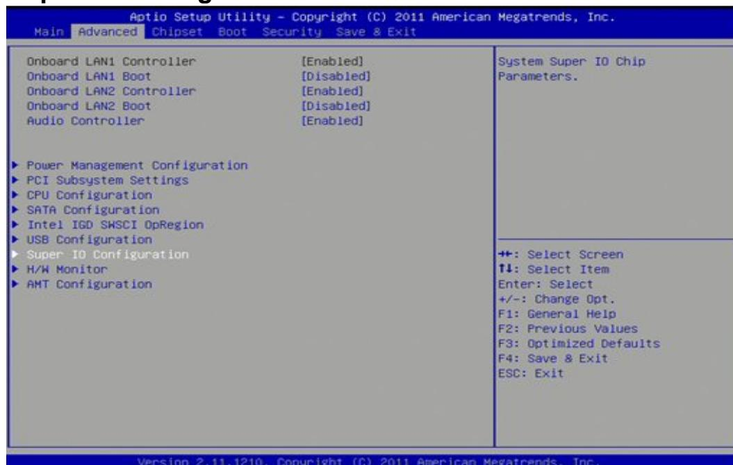
Select this option to set the IO Configuration function for onboard serial ports.
