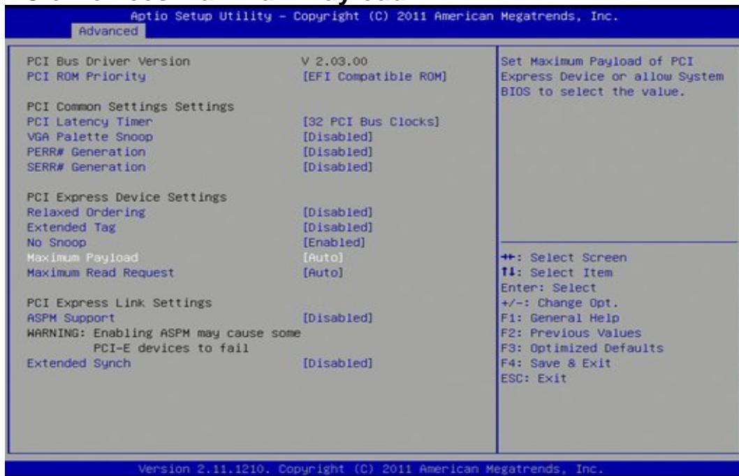
Select this option to set the Maximum Payload function (Auto).The maximum payload size defined by the PCI Express protocol and connected to send up to 4096 bytes.
