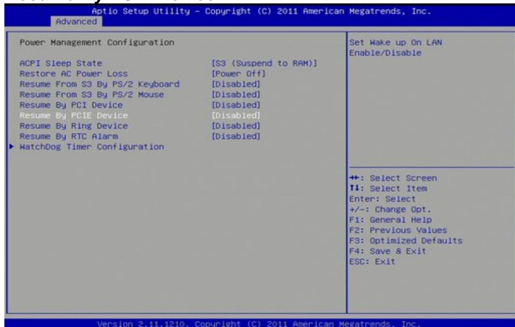
Select this option to disable or enable the PCIe device wake up function (Disabled).
