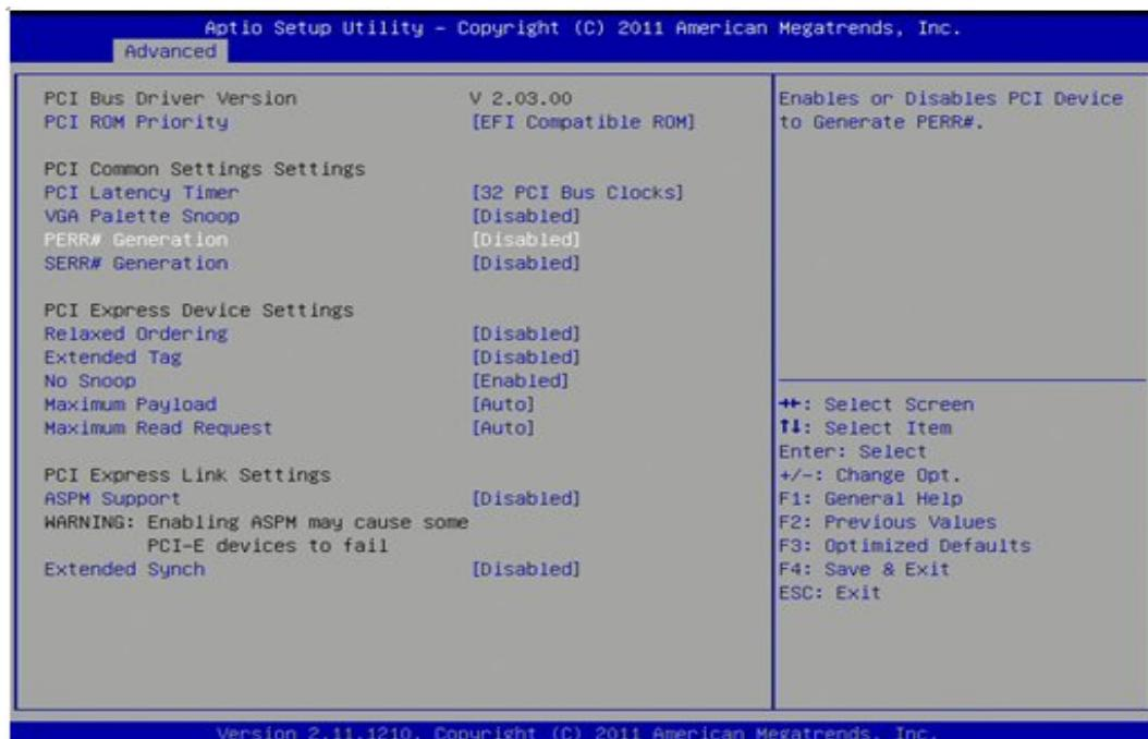
Select this option to enable or disable PERR# function (Default). When enabled the function allows PCI devices to generate PERR numbers.
