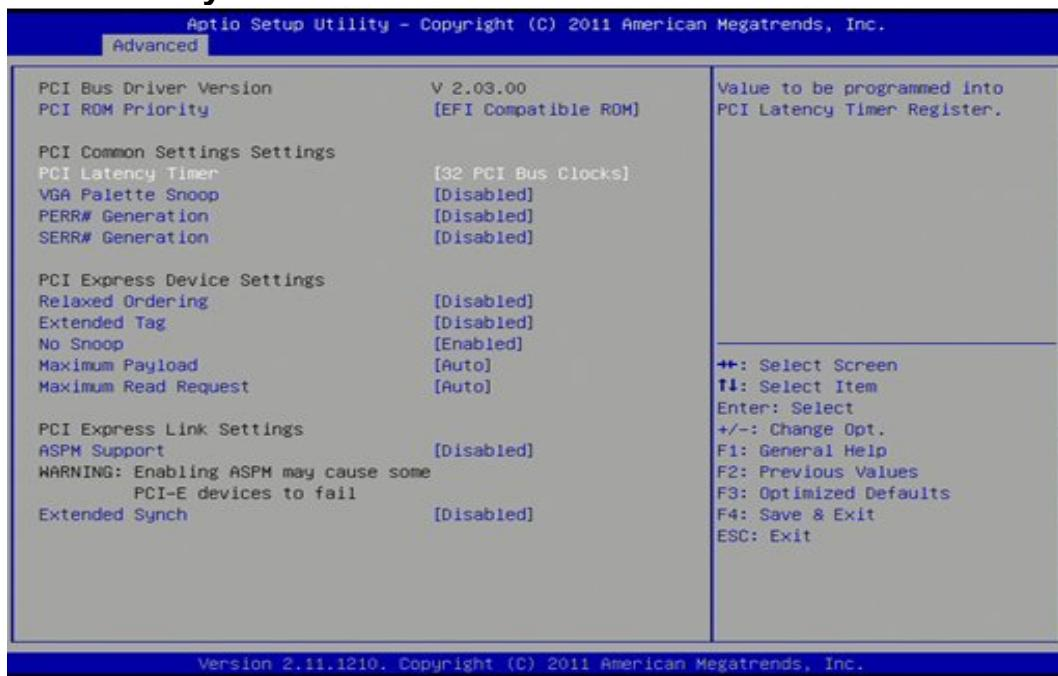
Select this option to set the PCI bus clock. Devices that operate in bus-master mode require a timer to limit the use of the PCI bus. This allows the use of the PCI bus by various devices. Setting a latency timer too low interrupts transfers unnecessarily, while setting a timer too high may cause a buffer overflow (devices requiring frequent bus access).
