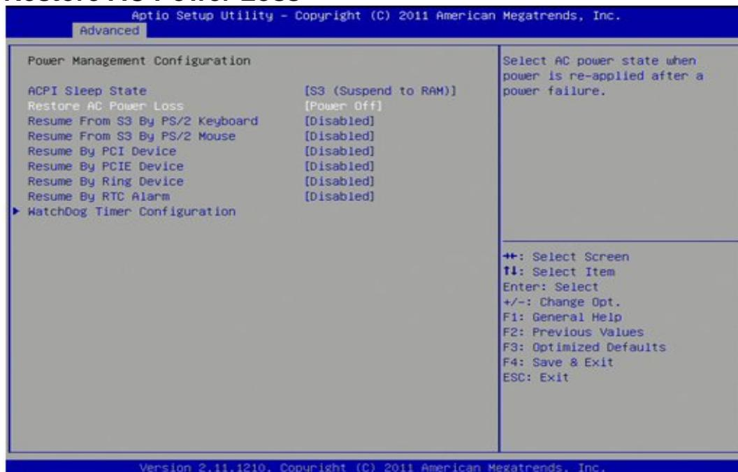
This menu specifies what state to go to when power is re-applied after a power failure (Power Off).
