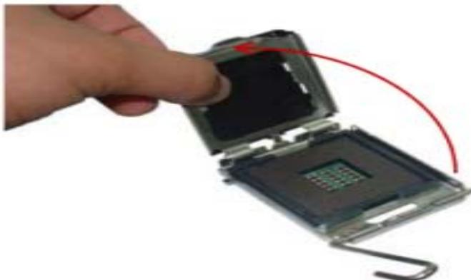
4. Push and remove the protective socket cover (plastic) from the load plate.
