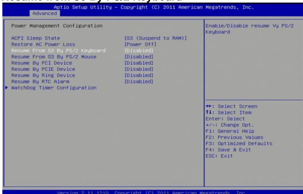
Select this option to enable or disable the PS/2 Keyboard wake up function from S3 mode (Disabled).
