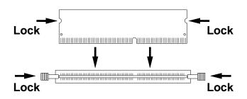
IMPORTANT: Ensure that the power supply is OFF during CPU and memory module installation.
