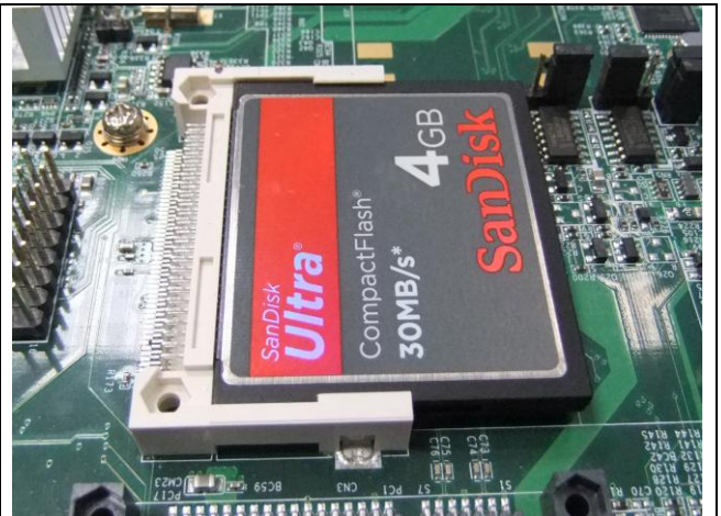
Fig. 7-2 Completion of CompactFlash Card connection
