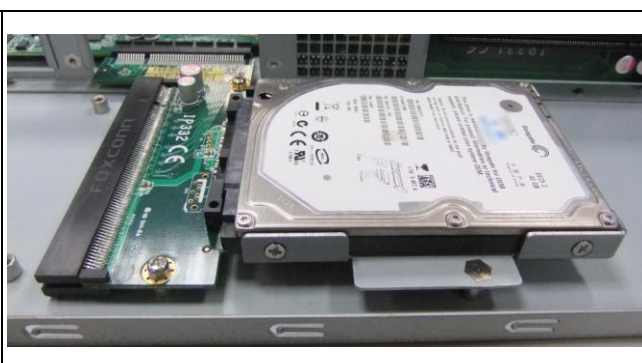
Fig. 9-4 Completion of HDD connection
