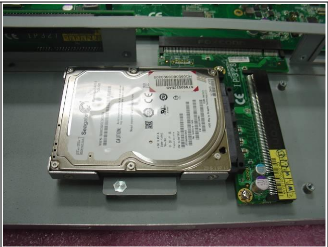
Fig. 9-4 Completion of HDD connection
