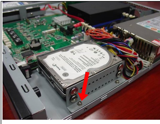
Fig. 10-3 Fix HDD bracket on chassis with four screws
