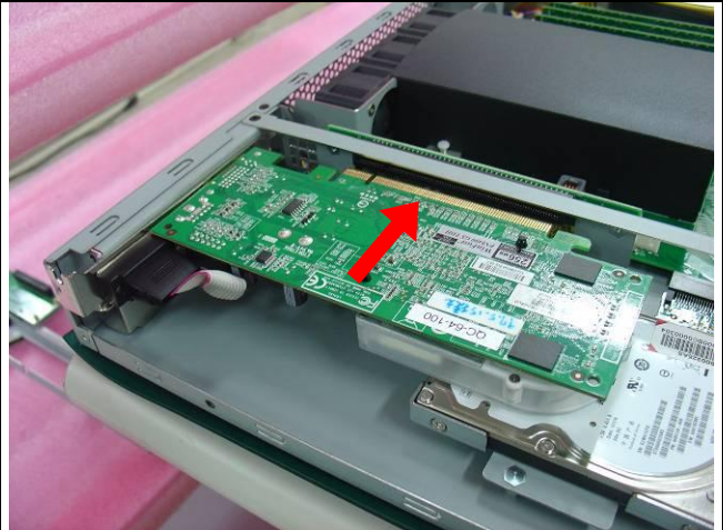
Fig. 11-2 Slide in PCI-e add-on card.
