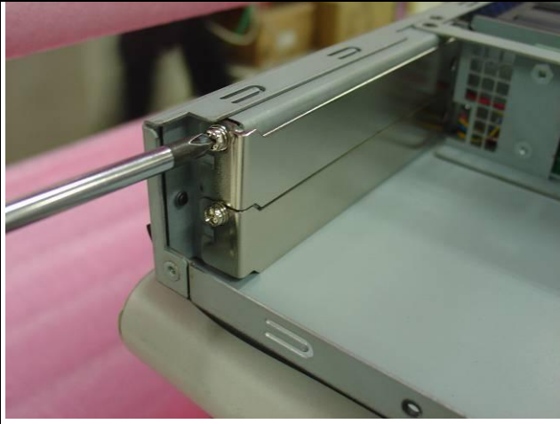
Fig. 11-1 Loosen screw on slot bracket.
