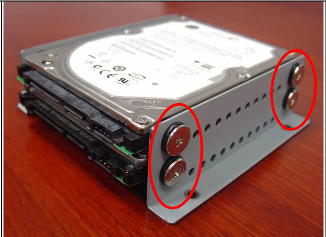
Fig. 10-2 Fasten the screws to lock 2.5" HDD bracket and bracket together.
