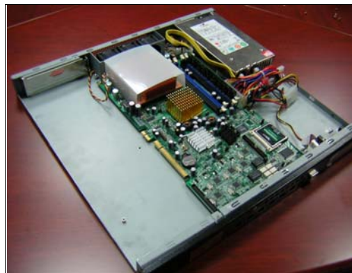
Fig. 7-3 Completion of Compact Flash Card connection
