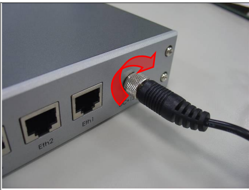
Fig. 9-1 Plug power connector into power jack
