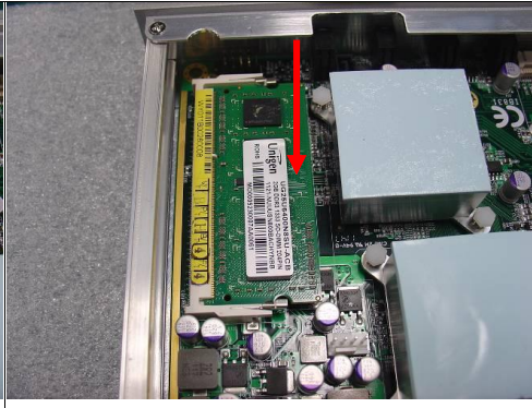
Fig. 7-2 Push down the memory module into socket
