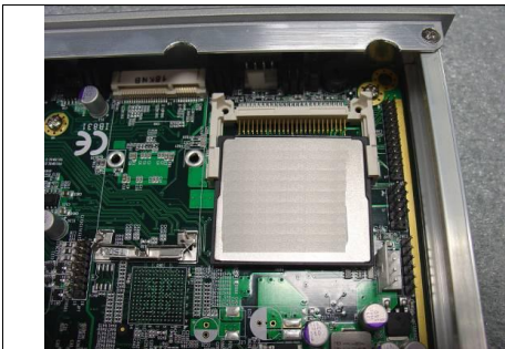
Fig. 6-1 Insert Compact Flash Card
