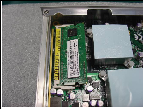
Fig. 7-1 Insert DDR3 SO-DIMM memory module
