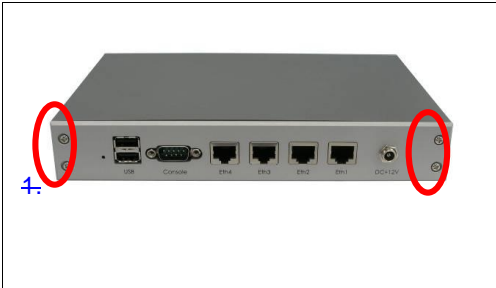
Fig. 5-1 Loosen four screws on back to remove the top lead. Keep the power cable locked on rear panel.
