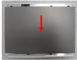
Fig. 5-2 The top lead can be removed from the base stand.
