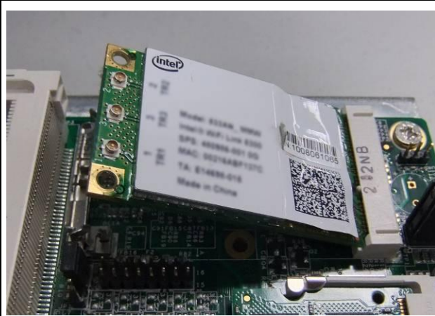
Fig. 9-1 Insert Mini PCI-e module (Supports USB signal only)
