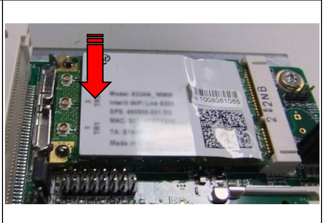
Fig. 9-2 Push down the module into socket
