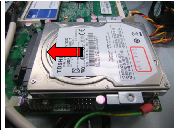
Fig. 8-3 Fasten both brackets on SSD with four screws
