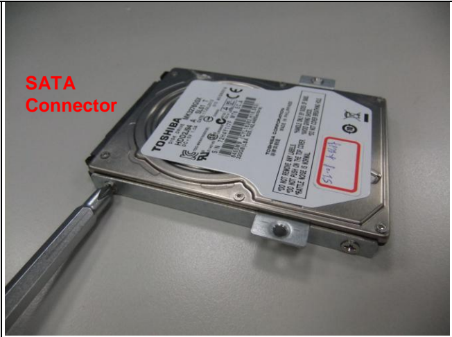
Fig. 8-2 Fasten brackets on SSD with four screws
