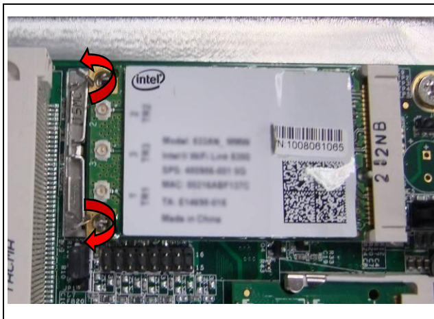
Fig. 9-3 Release two clips to remove module
