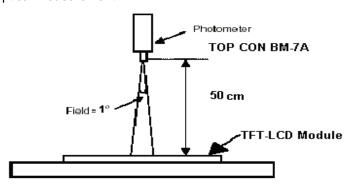
Note2: Measured at the central point of the LCD module and at the viewing angle of the  $\theta x=\theta y=0^{\circ}$
