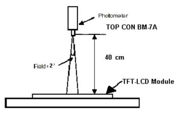
Note2: Measured at the center area of the panel and at the viewing angle of the  $\theta x = \theta y = 0^\circ$
