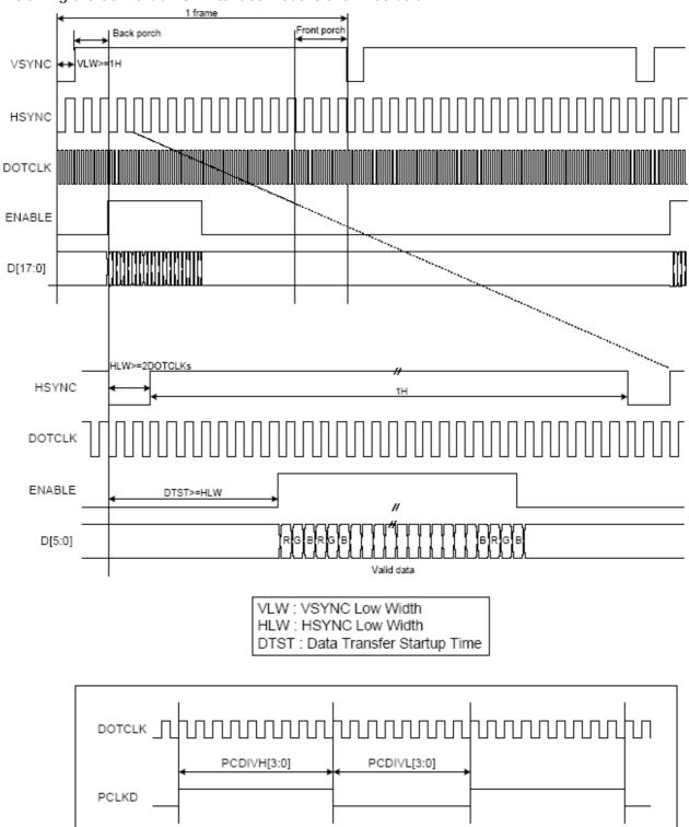
The timing chart of 18-bit RGB interface mode is shown as below.
