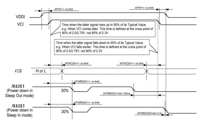
trPWRESX1 is applied to RESX falling in the Sleep Out Mode trPWRESX2 is applied to RESX falling in the Sleep In Mode
