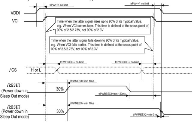
trPWRESX1 is applied to RESX falling in the Sleep Out Mode trPWRESX2 is applied to RESX falling in the Sleep In Mode
